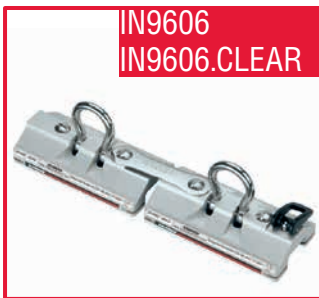
Three types of trolleys (single trolley for fall arrest system and double trolley for human suspension). The .CLEAR versions have natural coloration (showed above), the others are black anodized.
